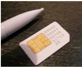
Figure 3: Picture of a smart card, here, a SIM card for use in mobile phones, size is 25x15 mm.
