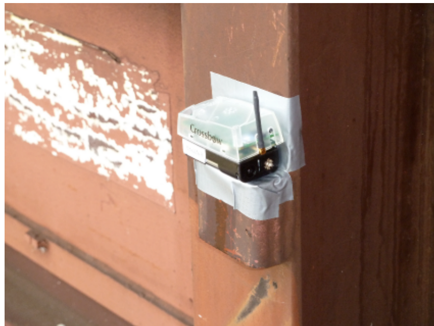
Figure 34 Box for sensor's protection
